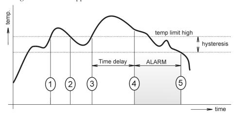
In Point 1 the temperature exceeded the limit. From this time, the time-delay is counting. Because at point 2 the temperature dropped below the limit value before the time delay expired, alarm was not set.
